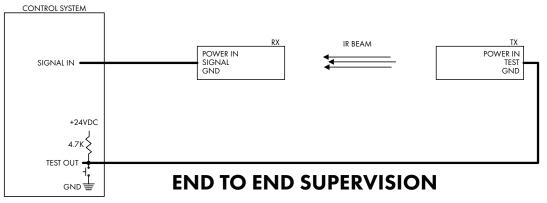
STEP 1: TEST OUT = FLOATING OR 24VDC, TURNS ON TX IR BEAM. STEP 2: CONTROL SYSTEM DETECTS SIGNAL IN ENABLED. STEP 3: TEST OUT = GND, TURNS OFF TX IR BEAM. STEP 4: CONTROL SYSTEM DETECTS SIGNAL IN DISABLED.
