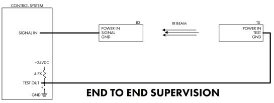
STEP 1: TEST OUT = FLOATING OR 24VDC, TURNS ON TX IR BEAM. STEP 2: CONTROL SYSTEM DETECTS SIGNAL IN ENABLED. STEP 3: TEST OUT = GND, TURNS OFF TX IR BEAM. STEP 4: CONTROL SYSTEM DETECTS SIGNAL IN DISABLED.
